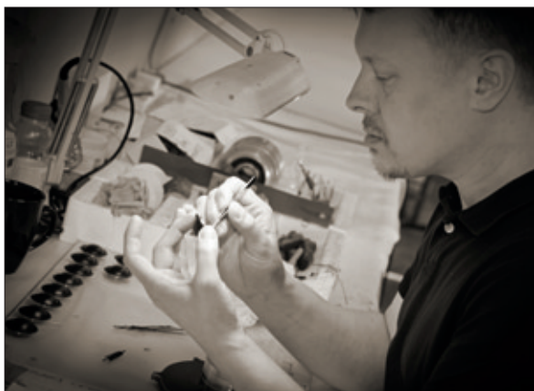
Filigree manual work: assembly of the carbon braces for the dome tweeter.
